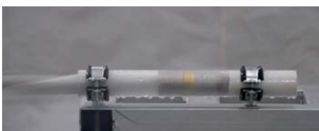
↗ Propulsion of the rotating lance during the cleaning process.
