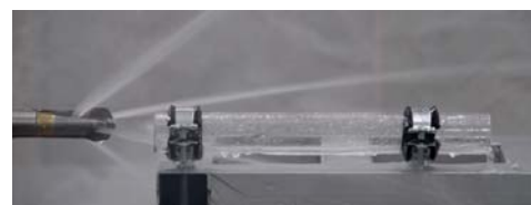
↗ The lance is retracted after cleaning the tube.
